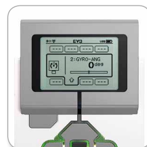
Port View with Gyro Sensor
